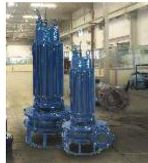
150HP Slurry Handling Pumps for TELCO
